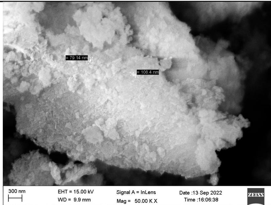
Fig. 2(b) SEM of  $\text{CoNiFe}_2\text{O}_4$
