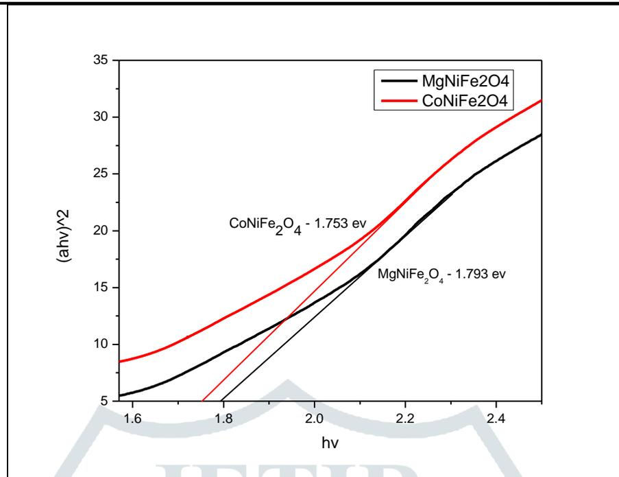
Fig. 4(b) UV-Visible spectrum of  $\text{MgNiFe}_2\text{O}_4$  &  $\text{CoNiFe}_2\text{O}_4$  for energy band gap
