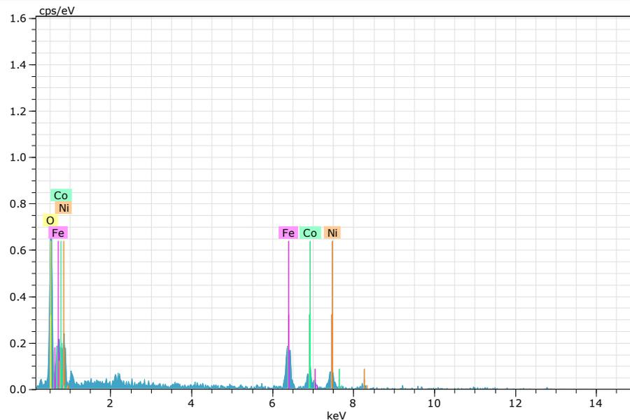
Fig. 3(b) EDS of CoNiFe<sub>2</sub>O<sub>4</sub>
