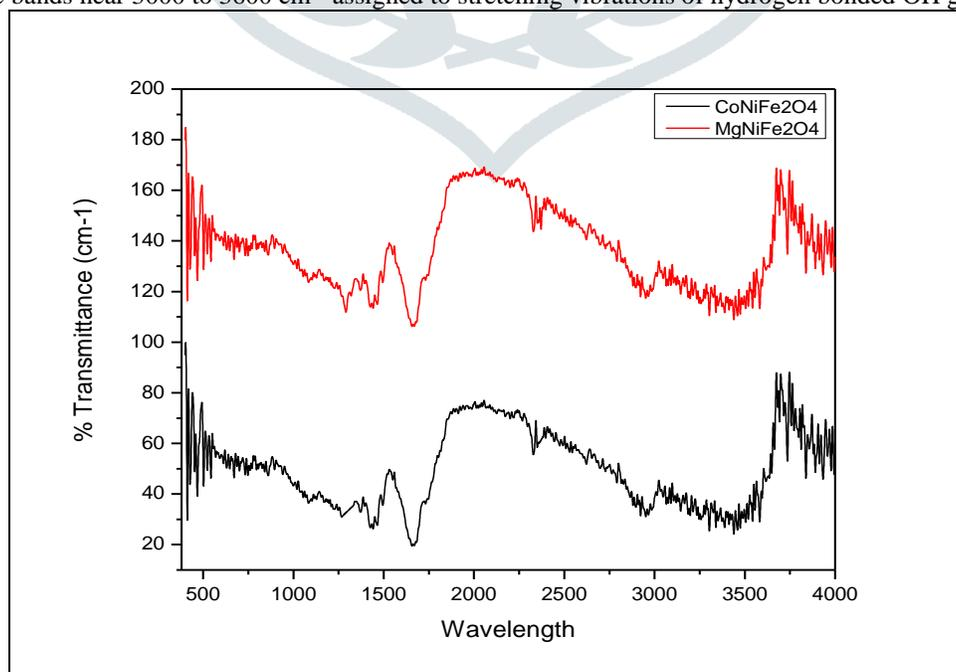
Fig. 5 FTIR spectrum of  $\text{MgNiFe}_2\text{O}_4$  &  $\text{CoNiFe}_2\text{O}_4$
