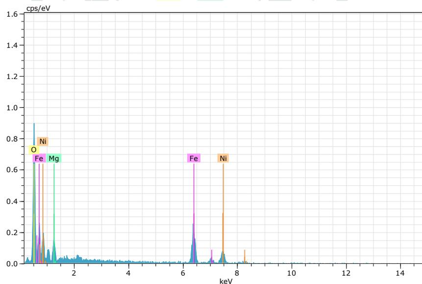
Fig. 3(a) EDS of  $\text{MgNiFe}_2\text{O}_4$
