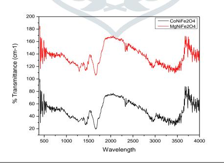
Fig. 5 FTIR spectrum of MgNiFe2O4 & CoNiFe2O4
