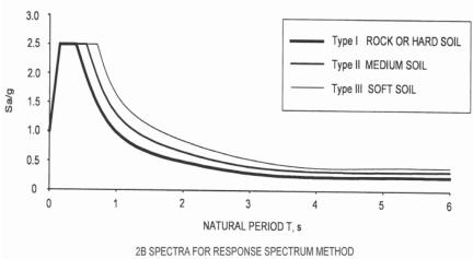
Figure 1. Response Spectrum curve IS 1983-2016
