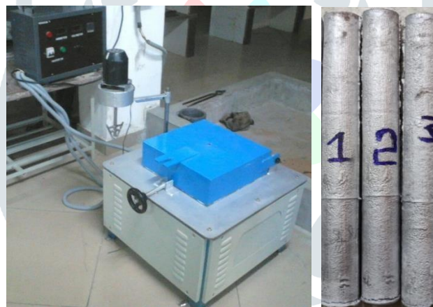
Figure 3. Stir casting setup and Casted Al7075 MMC rods
