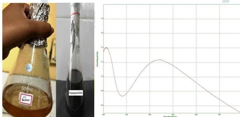
Fig.2a Synthesis of Nanoparticles Fig.2b Uv-Visble at 450nm
