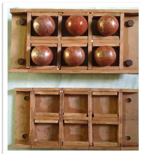
Fig. 2. Roller bearing base isolation prototype device
