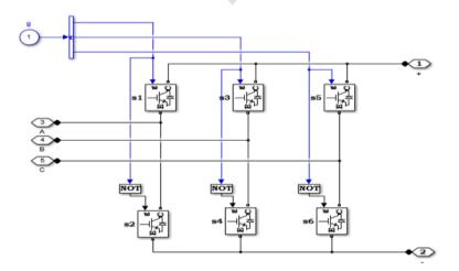
Figure 14. DVR's Power Circuit
