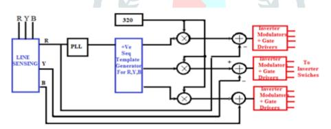
Figure 11. Block Diagram of a DVR's Control Strategy
