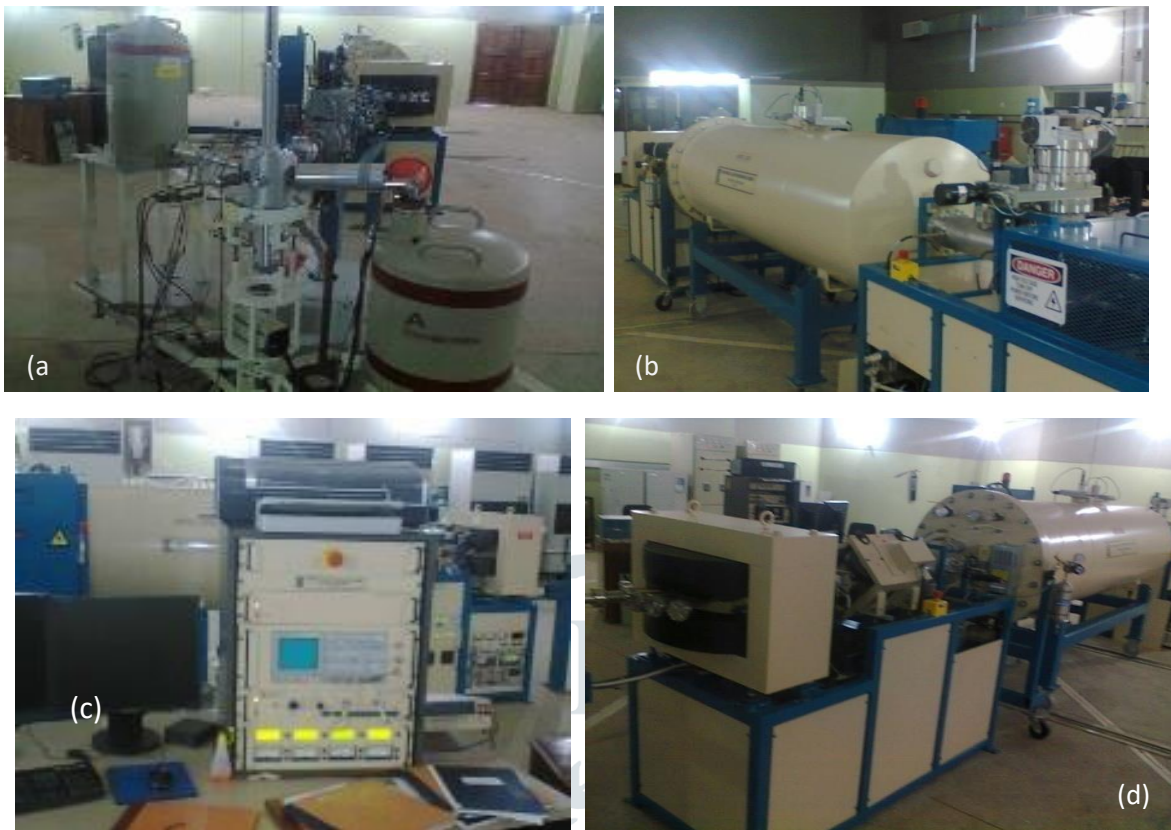
Fig.3.2: Set Up for Ion Beam Analysis with Tandem Accelerator (a – d)
