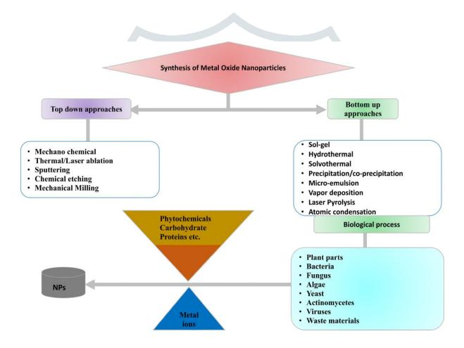
The bottom-up approach begins from the atomic level, through forming molecules. In the top-up approach, the scale of the resultant nanoparticles is larger, so that a mechanical process or the addition of acids is required to reduce the particle size. The top-down technique requires the use of complex & complicated instrumentation [13].
