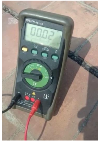
Fig 2.18 Amp value of small panel under direct sun
