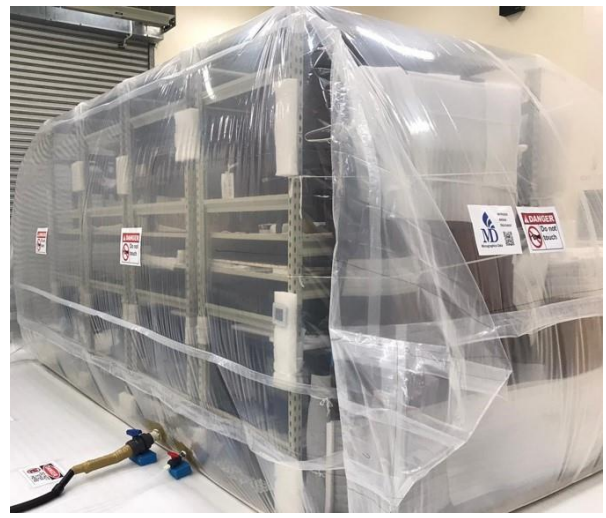
Fig. 4.2 Nitrogen Anoxia Treatment.
