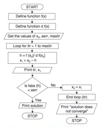
Figure 2: flow chart of Newton-Raphson method 3 RATE OF CONVERGENCE
