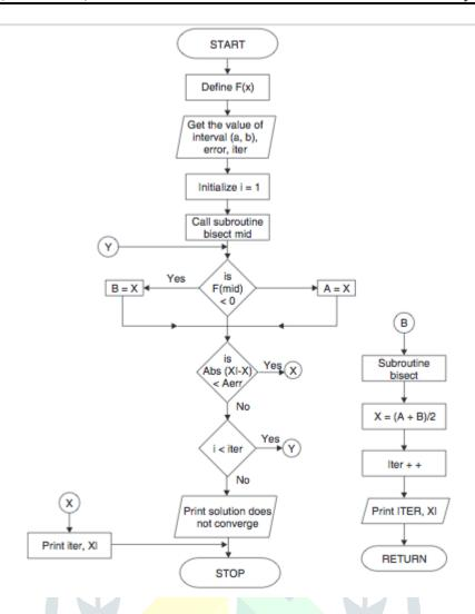
Figure 1: flow chart of Bisection method
