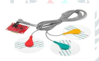
Connection between Arduino and AD8232 ECG Sensor: The AD8232 Heart Rate Monitor breaks out nine connections from the IC. We'll connect five of the nine pins on the board to Arduino. The five pins you need are labelled GND, 3.3v, OUTPUT, LO-, and LO+.
