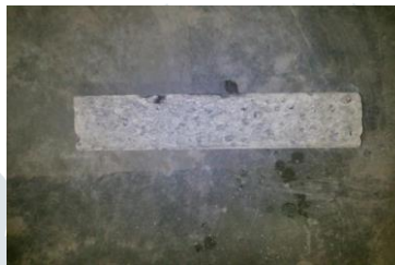
Fig2.6 Column specimen hand chiseled to make the surface rough
