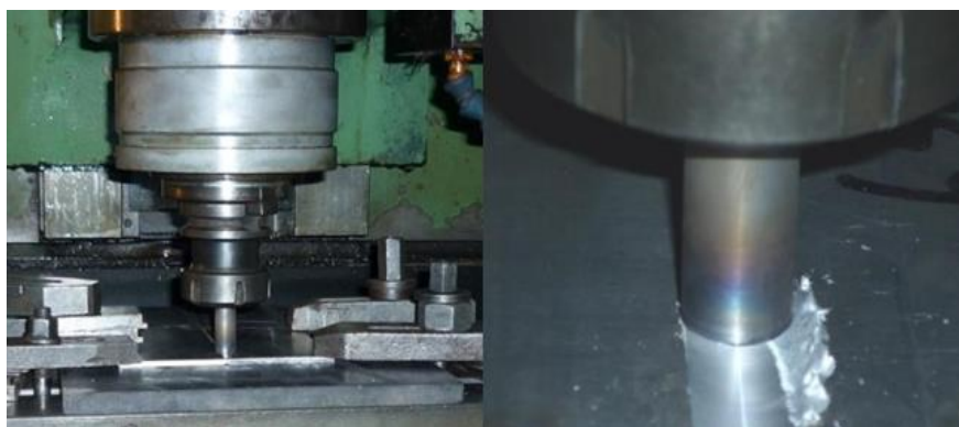
Fig. 6 Trial weld setup with cylindrical pin
