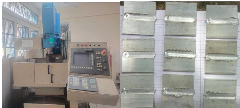
Fig. 7 CNC VMM and welded joints
