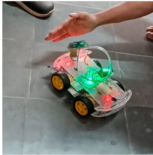
Figure 3. Obstacle identifying and reorient its path of the Robot
