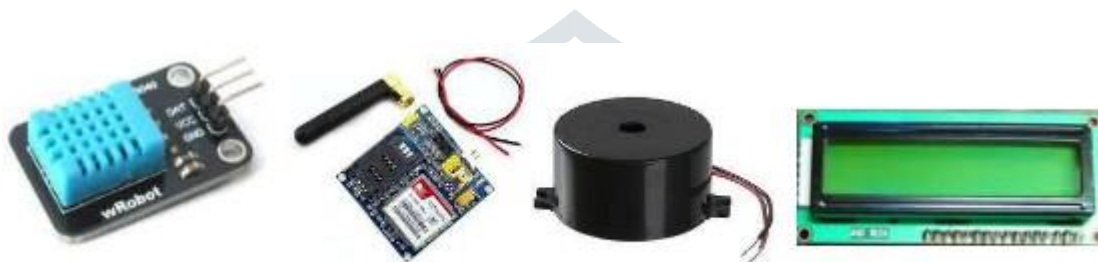
Figure2. DH-11 sensor, Buzzer, GSM modem (Sim900), Liquid crystal display unit (LCD)
