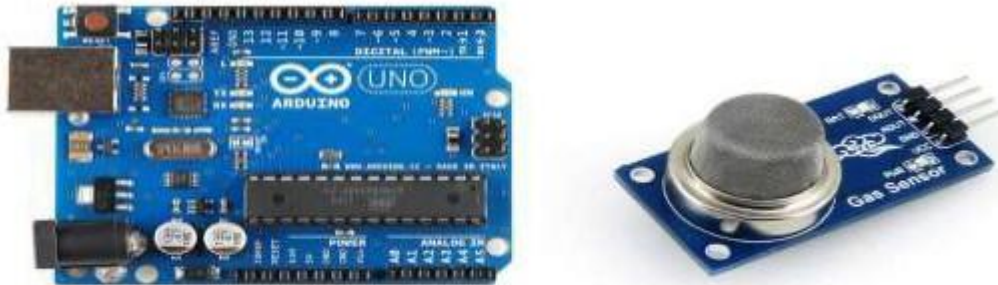
Figure1. Arduino UNO microcontroller and MQ-6 Sensor
