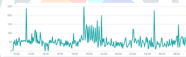
Figure 13: graph of IPS logs during port scanning and brute-force attack
