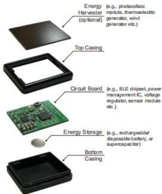
Fig. 5. An illustration of generic hardware components of BLE beacon.
