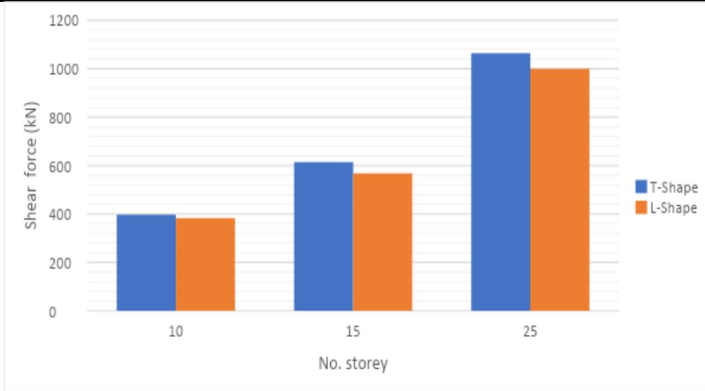
**Fig. 4.: Comparison of shear force under seismic loading condition**
