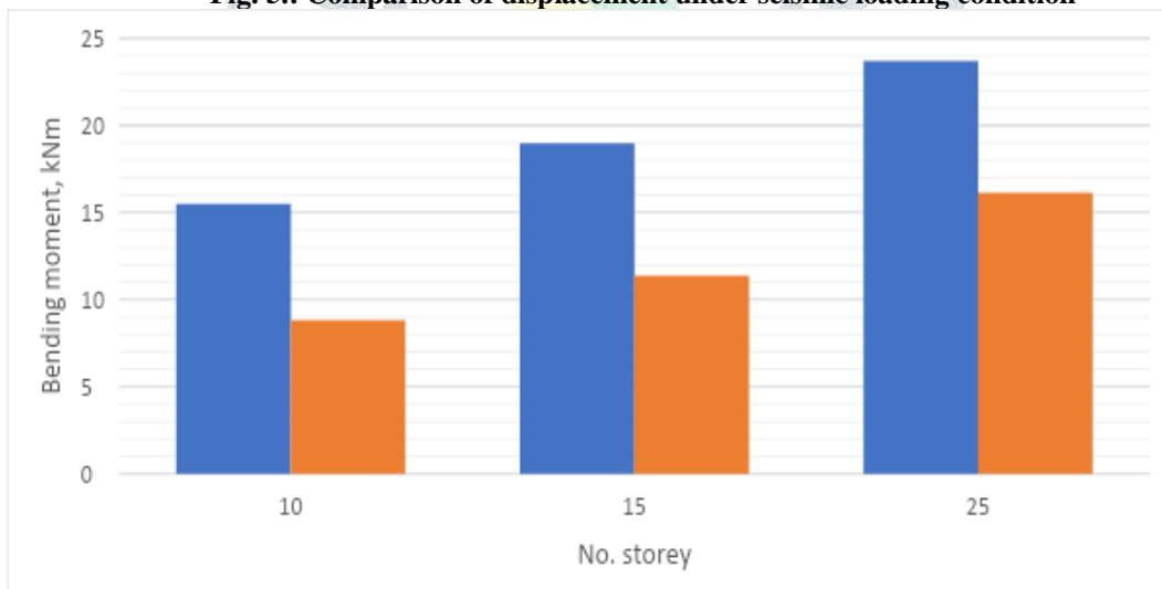
**Fig. 6: Comparison of bending moment under seismic loading condition**
