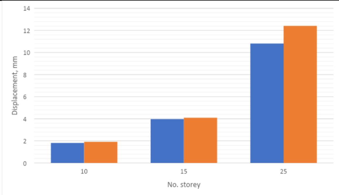
**Fig. 9: Comparison of displacement under wind loading condition**
