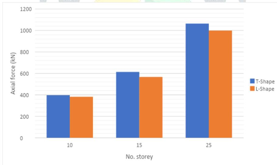
**Fig. 3: Comparison of axial force under seismic loading condition**
