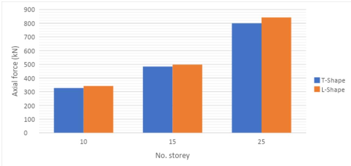
Fig. 7: Comparison of axial force under wind loading condition
