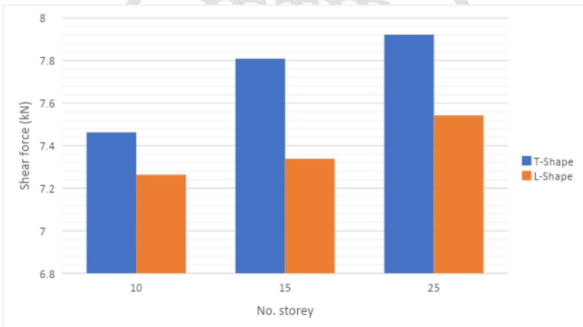
Fig. 8: Comparison of shear force under wind loading condition
