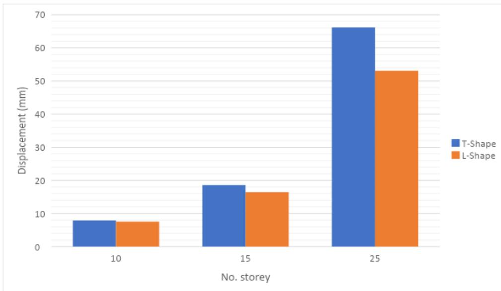
**Fig. 5.: Comparison of displacement under seismic loading condition**
