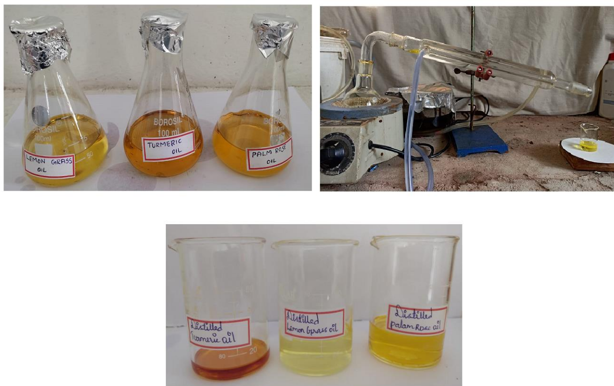
Figure 1: Diagram representing the extraction action of essential oil by using distillation process from Lemon grass ( Cymbopogon flexuosus ), Turmeric oil ( Curcuma longa ) and Palmarosa ( Cymbopogon martinii )
