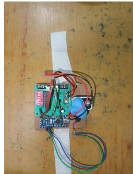
Fig-6: Wrist band with RF receiver and vibrator
