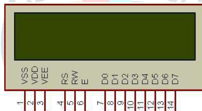
Figure 10 LCD Module with Pin Description
