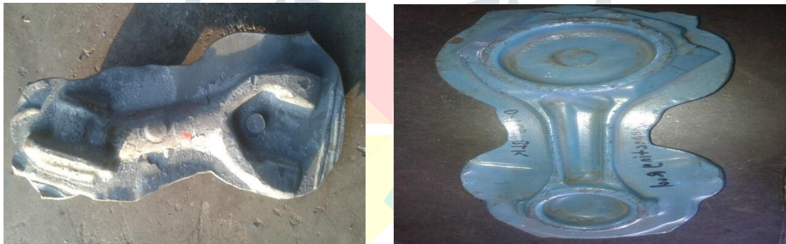
Fig 08 Flash Formation Around Job.
