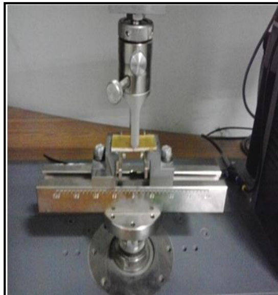
Fig.6 Specimen positioning in three-point bend test on UTM
