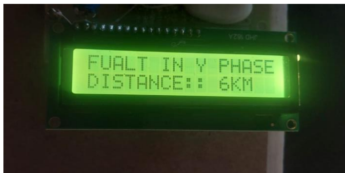
Fig 3(b) LCD displaying fault
