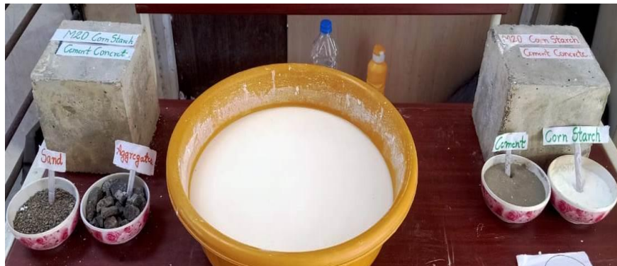
Figure No: 1, "Ingredients of corn starch concrete"
