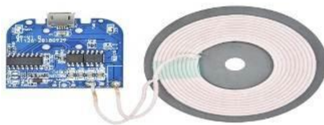
Fig 5c) Wireless Charging Module
