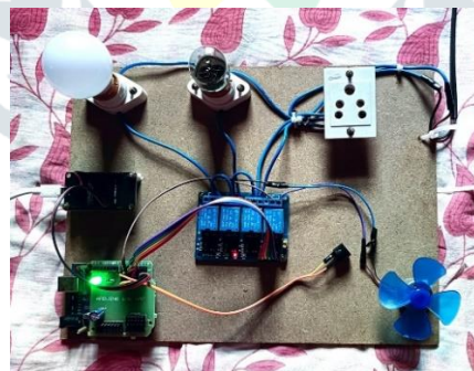
Fig 6.7: Circuit with voice command Lamp off
