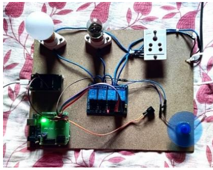
Fig 6.4 : Circuit with voice command Fan on
