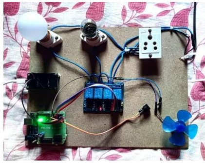
Fig 6.9: Circuit with voice command Socket off
