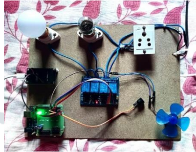
Fig 6.5 : Circuit with voice command Fan off
