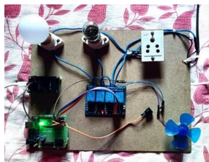
Fig 6.8:Circuit with voice command Socket on
