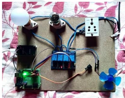
Fig 6.3 : Circuit with voice command Light off
