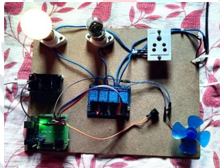
Fig 6.2 : Circuit with voice command Light on
