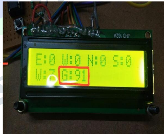
Fig 21: LCD displays amount of Air Pollution Presence
