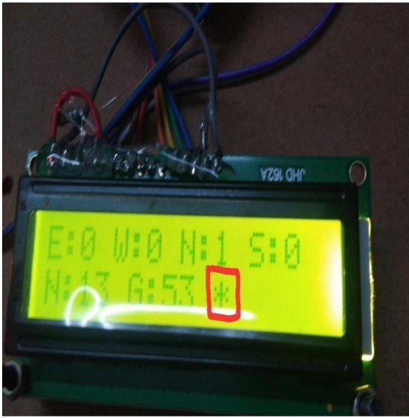
Fig 10: Identification for Emergency vehicle is near -"*"
