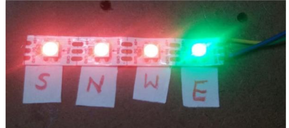
Fig 14: LED displays green at East direction
