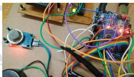
Fig 20: Interfacing of ARDUINO with GAS Sensor
