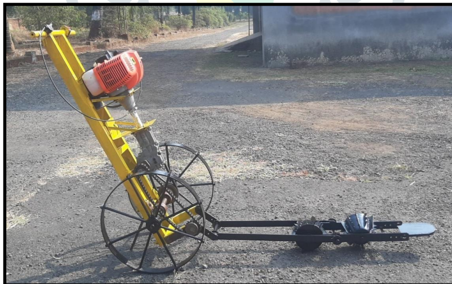
Plate no. 1 Developed reciprocating type of power operated conoweeder
