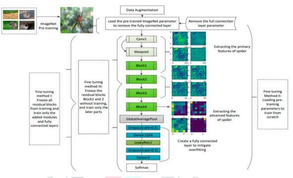
Fig. 1: Block Diagram of Proposed Attention-based VGG-16 Model
