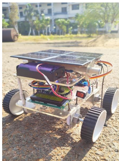
Fig: Solar Top-Roof Charging System
