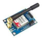
**Figure 5: GSM Module**
