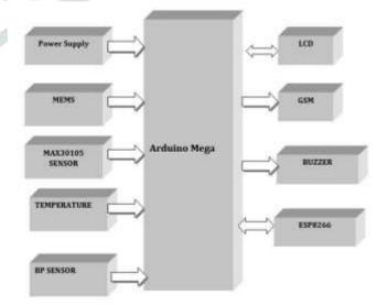
Figure 11: Block Diagram
