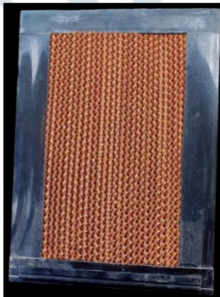
Fig. 3.1 Honeycomb Mesh Layer on Aluminium Frame Body
