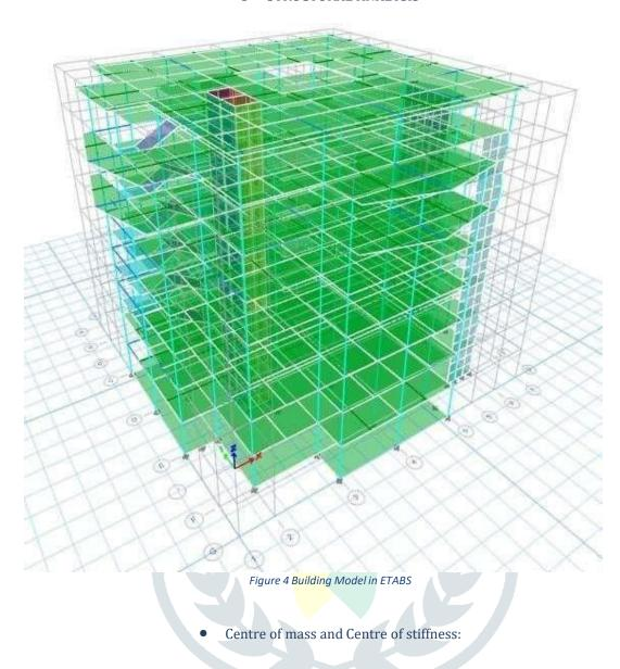
Centre of mass of each storey was calculated manually, along with the center of rigidity for thepreliminary architectural plan. Additionally, these values were generated from the ETABS model, and compared. Eccentricity thus observed was used in determining changes, to structural configuration.
