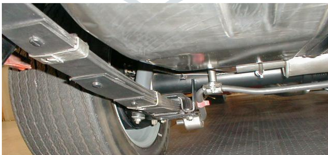
Fig 2. A traditional leaf spring arrangement.
