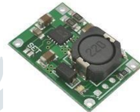
Fig: Charge Controller
