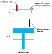
Exhaust valve is open and inlet valve is closed piston starts to move
