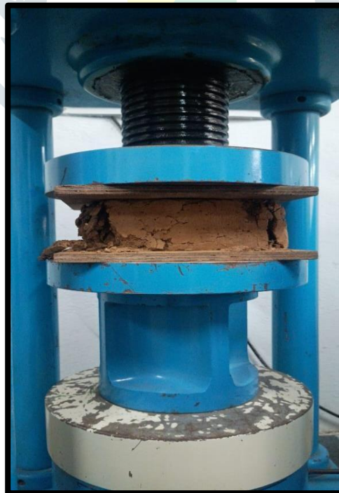
Fig 5.2: Compressive Strength of Bricks with cement content
