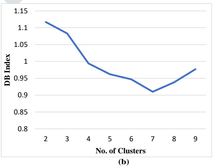
Fig. 11: No. of classes vs Davies Bouldin for (a) K-mean and (b) Auto-Model
