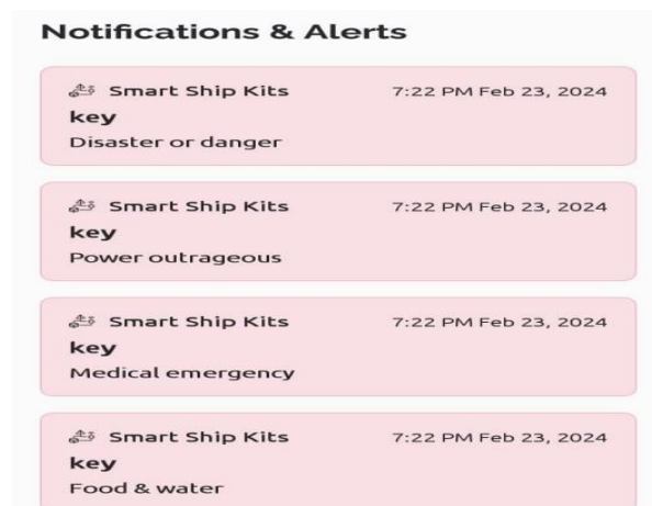
Figure 13. Blynk App outputs for keys used in boat sinking alert system
