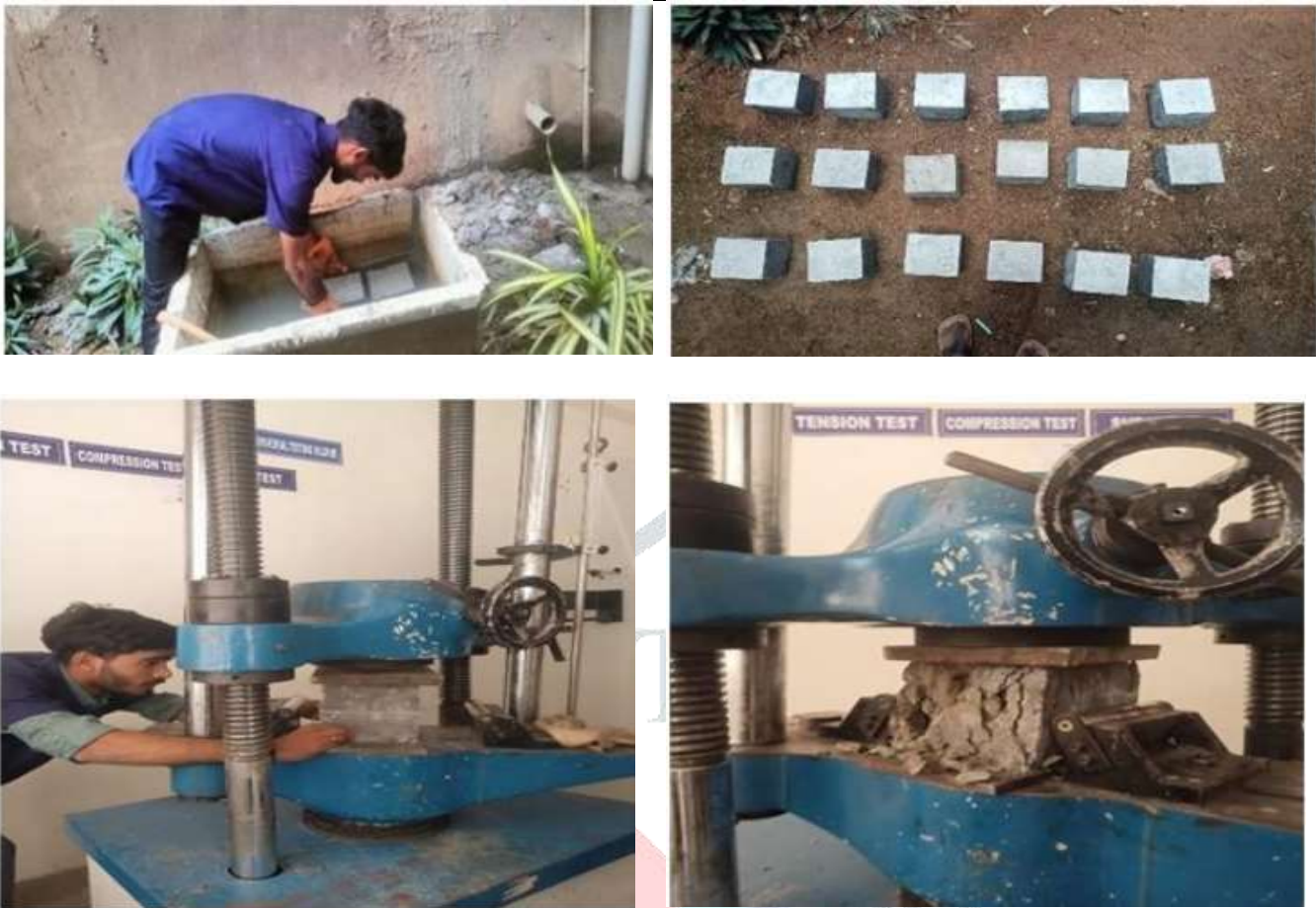
Fig 1: Experimental testing process starting from sample preparation to compressive testing.
