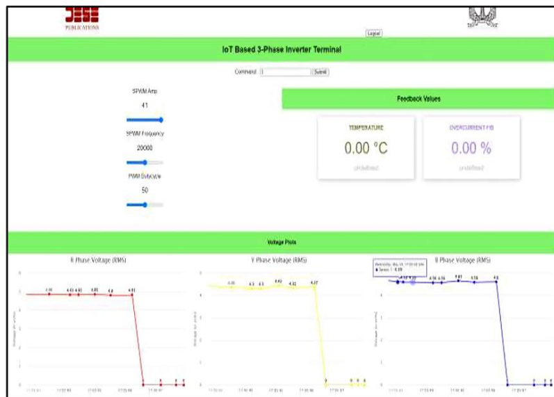
Figure 11: SPWM Operation Feedback @ 20 kHz 11 Amp default SPWM
