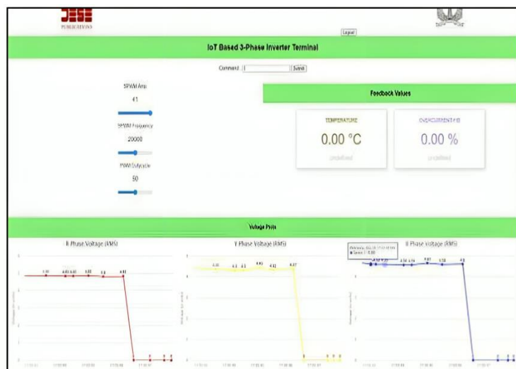
Figure 12: Stop by giving command 3 while running @ default SPWM.
