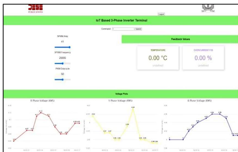
Figure 10: SPWM Operation Feedback @ 20 kHz 41 Amp default SPWM
