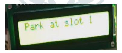
Fig 5: Lcd Showing parking Allotment
