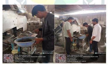
Step No 4: Compacting the material
