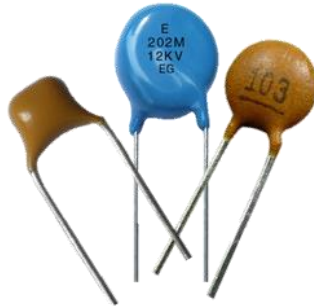
Fig no :5.5 Capacitors
