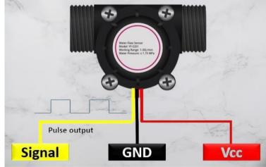
when the water is continuously flowing through it, if the reading speed is high then the output is high, and vice versa [6].
