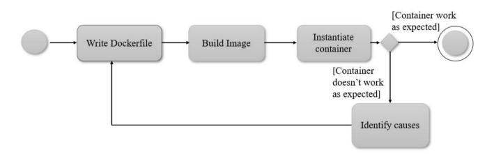
Fig1: Motivational example of a workflow when developing a Dockerfile.
