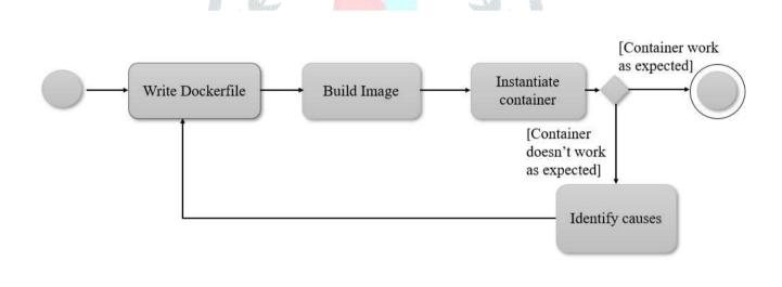
Fig1: Motivational example of a workflow when developing a Dockerfile.
