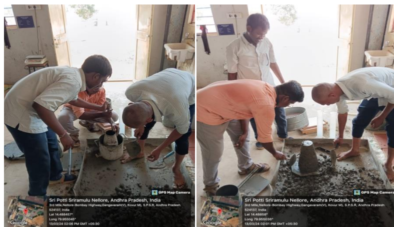
Fig 3.1.2 Workability tests conducted for concrete composition
