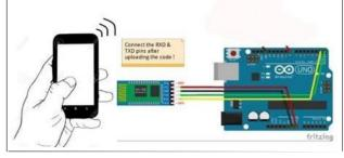
Fig. 7. Connection of bluetooth module to arduino uno
